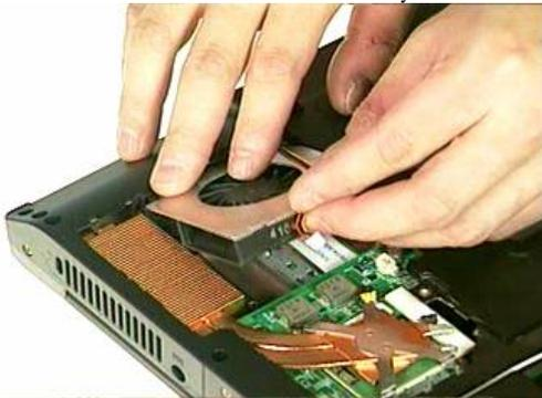
(f). Remove the 4 screws upon the CPU module (No.5 ~No.8)
