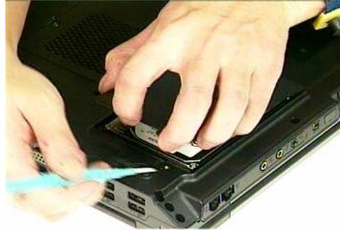
(b). Pull out the hard drive and lift the hard drive away by 2 hands.
