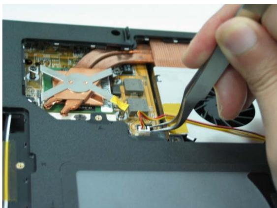
(d). Remove the 2 screws aside the CPU fan
