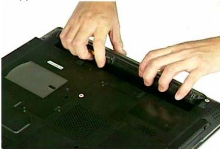
(c) Slide the battery latch to unlock. Firmly slide the other latch to the top and remove the battery.
