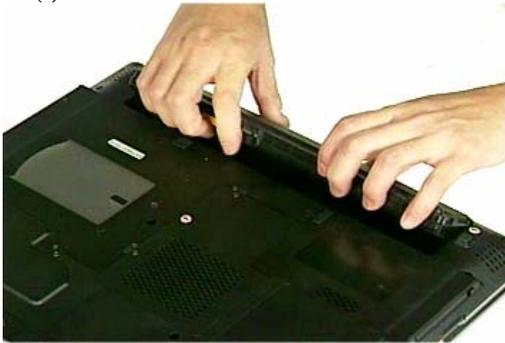
(b). Slide the battery latch (No.1) to unlock.
