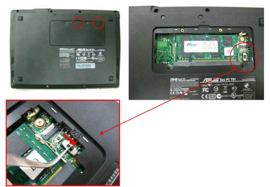
2. Softly open the two latches to pop the memory module up at 45 degree angles then remove the memory at that angle.
